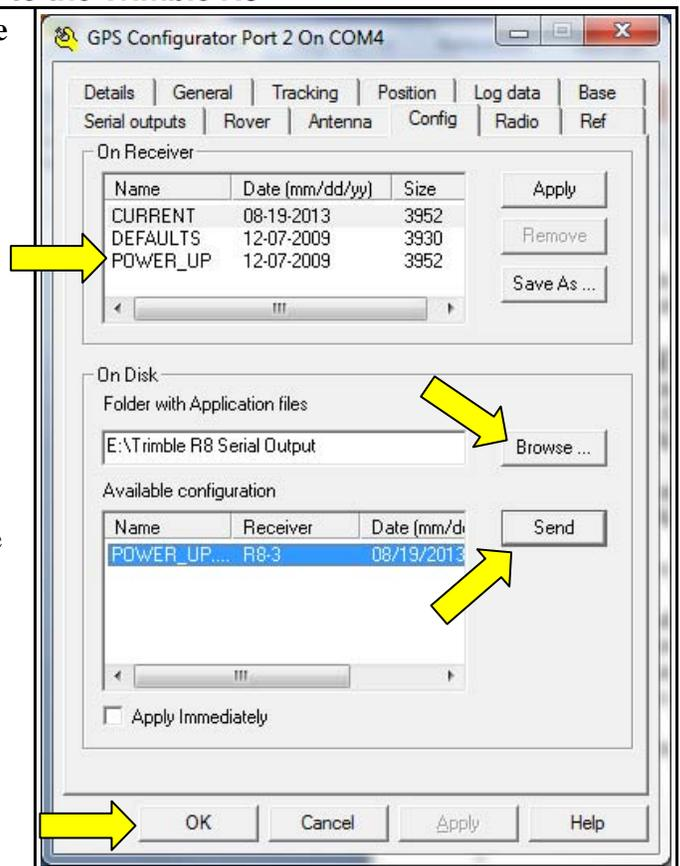
Now when you start the Trimble R8 it will load the settings in the **POWER\_UP.CFG** file and operate as it was when the **POWER\_UP.CFG** file was created.
