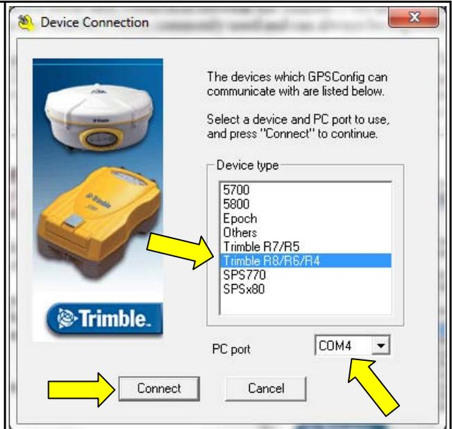
GPS Configurator will establish a connection with the Trimble R8 and display a dialog as shown at right. This time the **Details** tab came up first; your results may vary.
