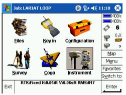
Once the Survey has begun you will see a message showing "Building Base File" once this has completed press "Accept". The Survey has been started, we are ready to begin measuring points or we can go directly to site calibration in the Survey
