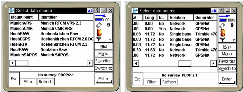
Figure 4.2 Selection field (first view and right-scrolled view) at a Trimble ACU running Survey Controller v. 10.7
