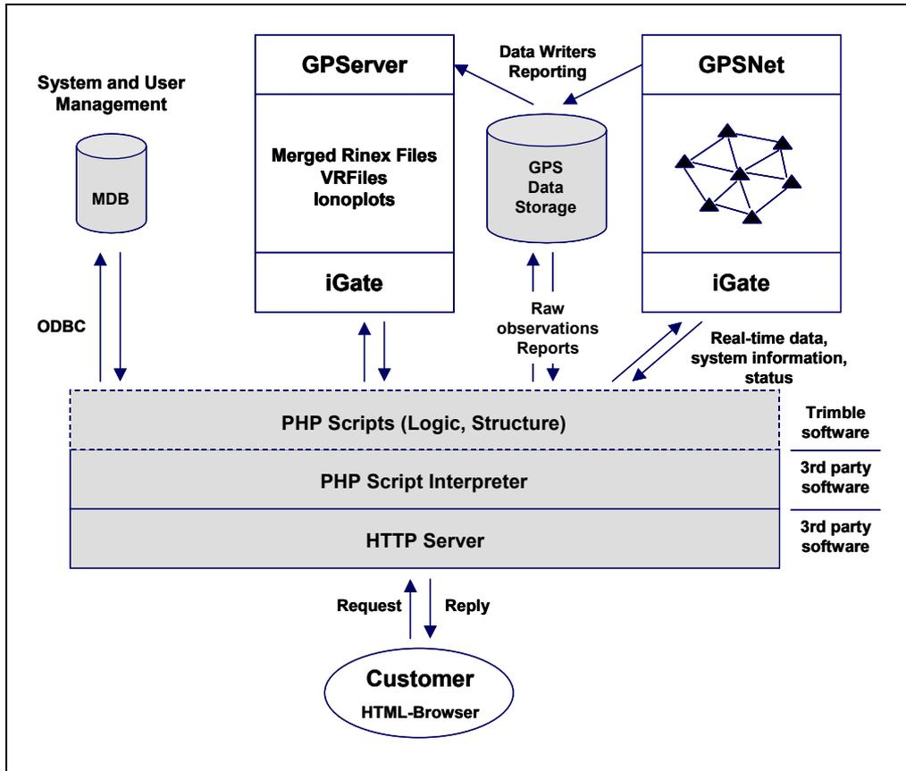
Figure 3.1 System components of a GPServer web server system
